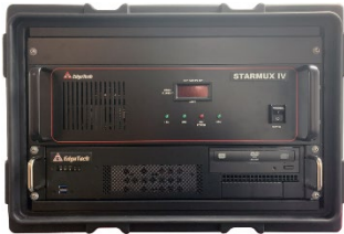
RACK MOUNT (STARMUX IV DL AND 2U COMPUTER IN 6U CASE)
