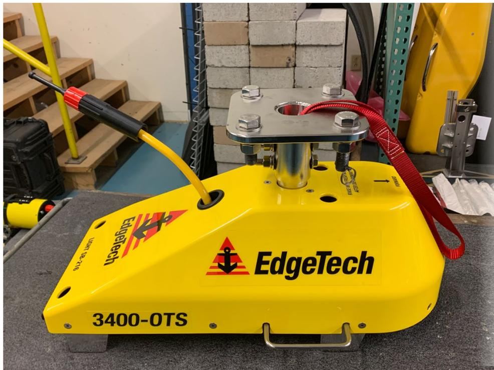
*Figure 4-51: 3400 Light and Ultra-Light Adaptor Flange Installation - Pole-Mount Adaptor Flange Mounted*
