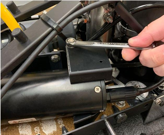
*Figure 5-12: 3400 OTS Light and Ultra-Light Electronics Bottle - Mounting Block to Electronics Bottle Mounting Bolt Unthreading*
