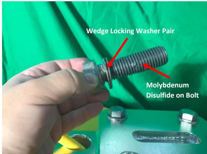
Figure 4-26: Forward Dorsal Bolt Locking Washer and Molybdenum Disulfide Coating
