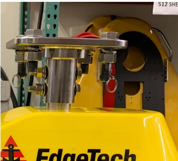
*Figure 4-55: 3400 Light and Ultra-Light Adaptor Flange Plate Screw Assembly Locations*
