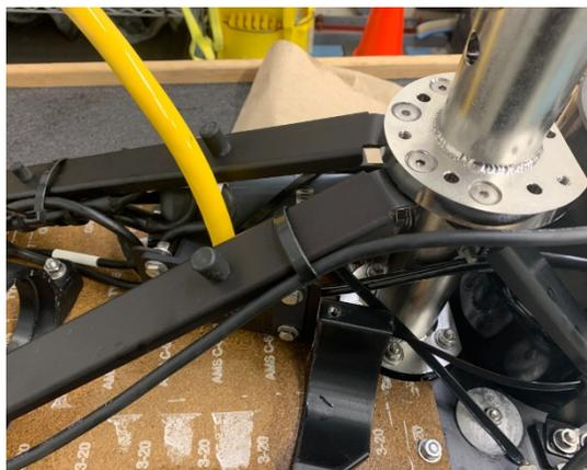
Figure 5-8: 3400 OTS Light and Ultra-Light Transducer Installation - Cable Ties
