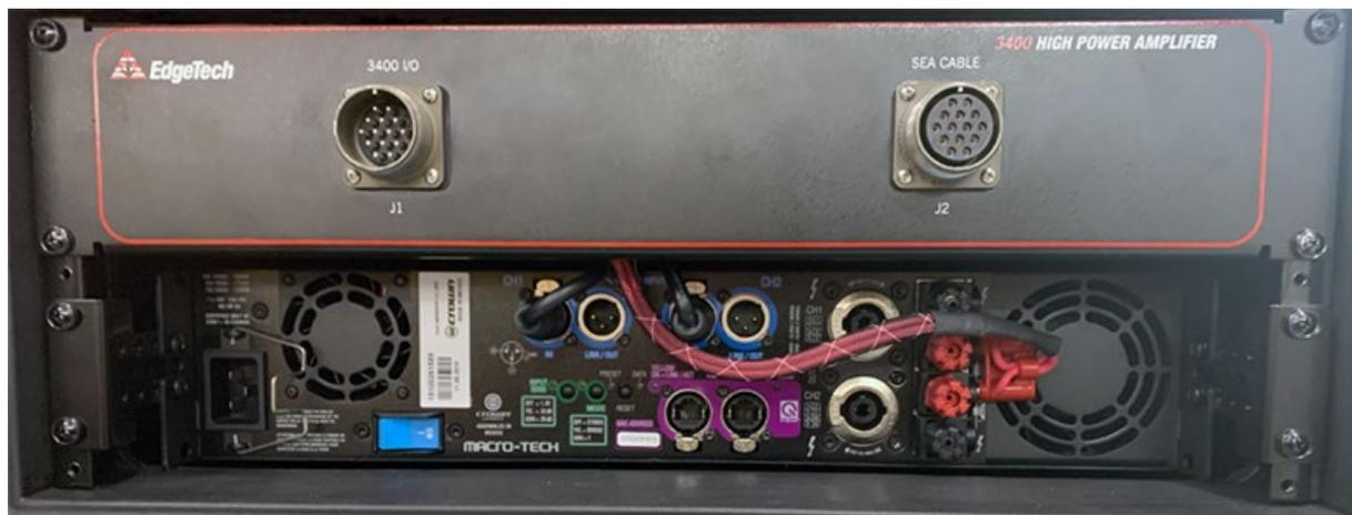
*Figure 3-13: Back Panel Amplifier and Connector Panel*
