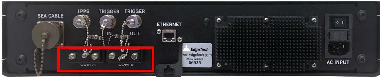
Figure 4-42: 3400 Topside Serial Port Navigation Connection
