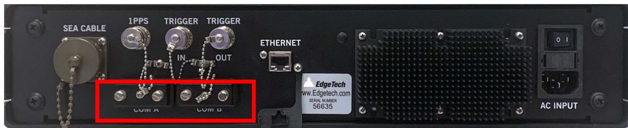
*Figure 4-1: 3400 Topside Serial Port Navigation Connection*
