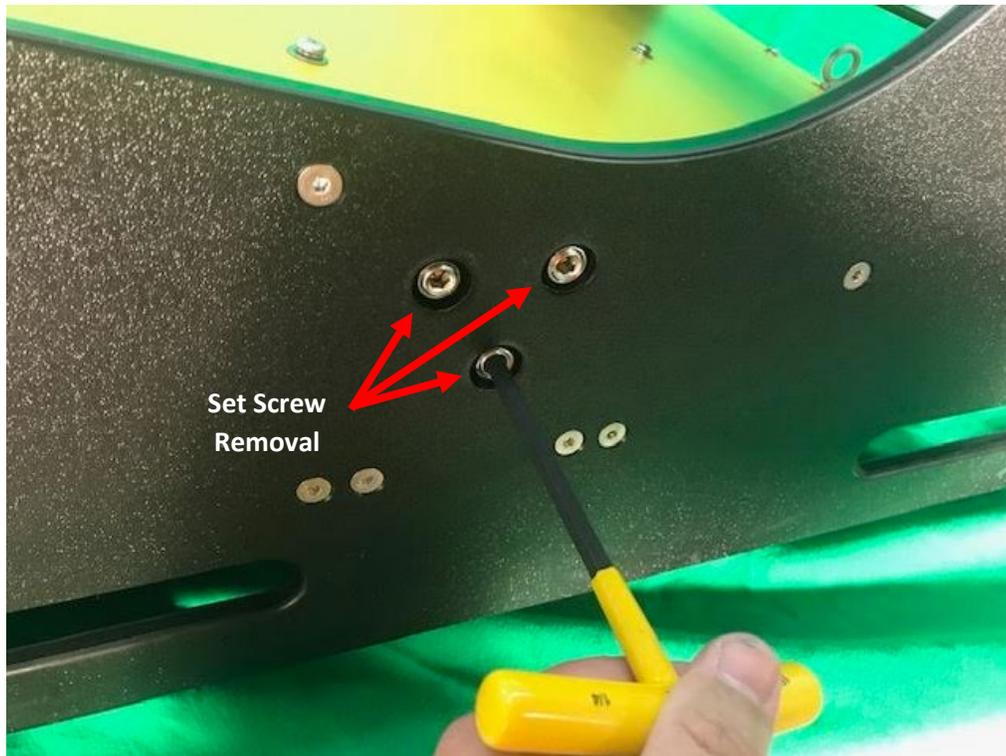
*Figure 4-24: Port and Starboard Set Screw Removal*
