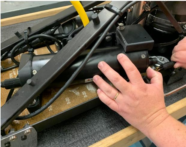
*Figure 5-10: 3400 OTS Light and Ultra-Light Electronics Bottle-Cable Disconnection Figure 1*
