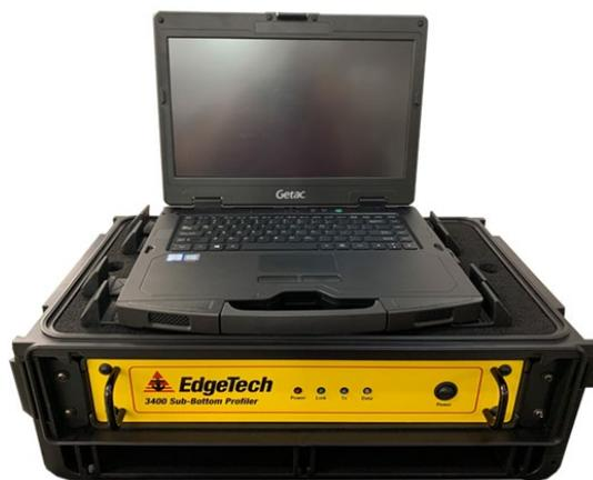
*Figure 1-9: Deployed 3400 Rackmount System*
