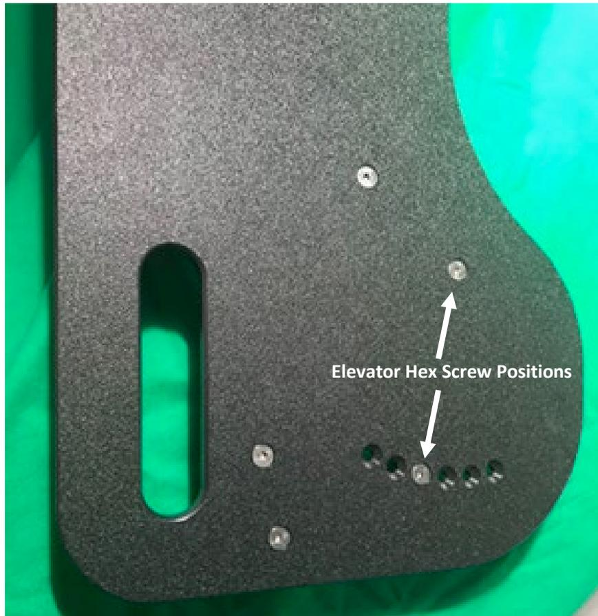
*Figure 5-2: Elevator Hex Screw Positions*
