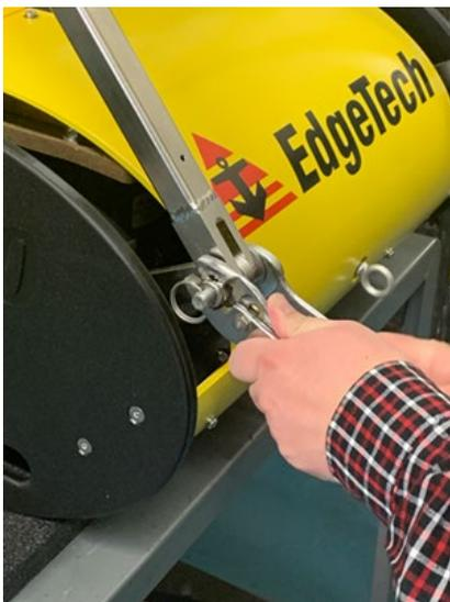
Figure 4-12: Loosening Bridle Elbow
