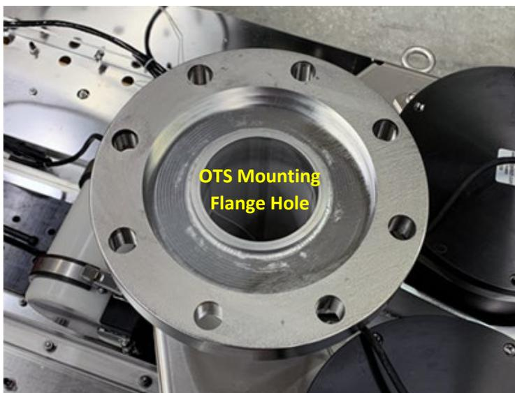
Figure 4-38: OTS LF Mounting Flange
