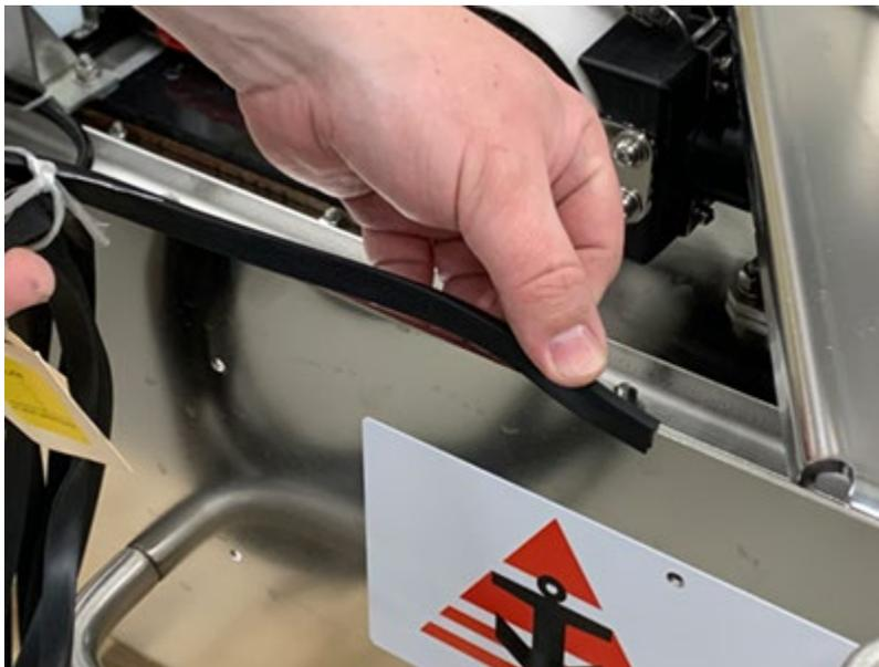
*Figure 4-35: 3400 OTS LF Rubber Trim Installation*
