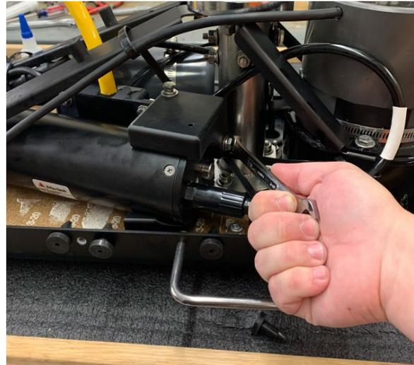
*Figure 5-13: 3400 OTS Light and Ultra-Light Electronics Bottle - Mounting Block to Electronics Bottle Bolt Unthreading*
