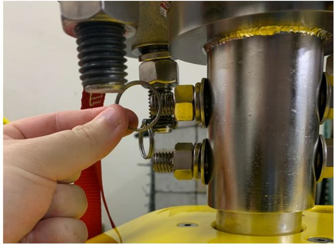
*Figure 4-50: 3400 Light and Ultra-Light Adaptor Flange Installation - Split Ring Installation*
