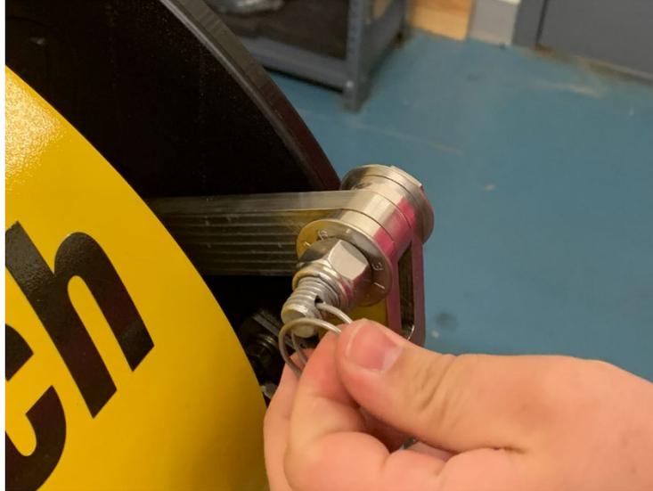
*Figure 4-17: Bridle Removal: Split Ring Removal*
