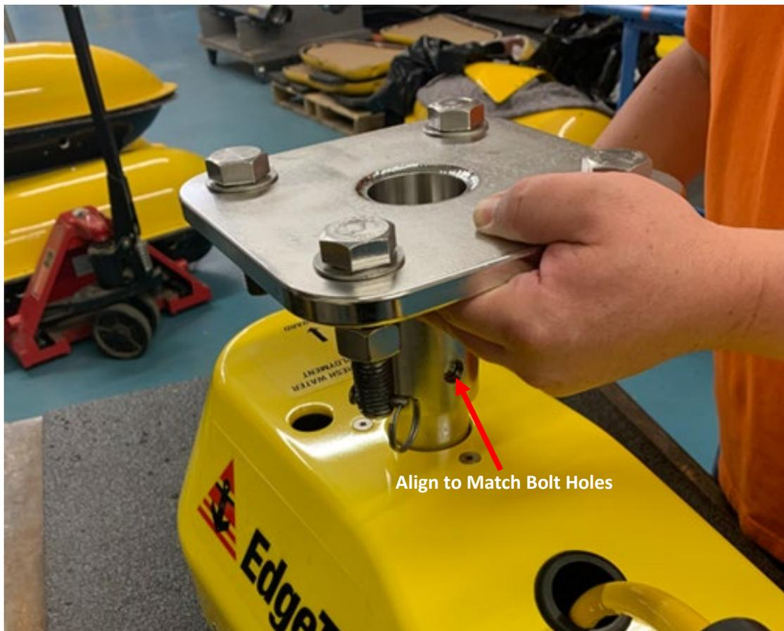
Figure 4-45: 3400 Light and Ultra-Light Adaptor Flange Installation - Adaptor Installation and Alignment
