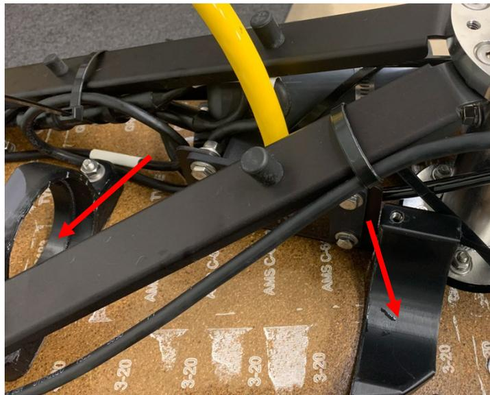
*Figure 5-14: 3400 OTS Light and Ultra-Light Vehicle Bottle Mountings*
