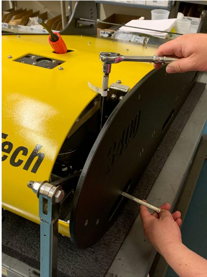
*Figure 4-16: Bridle Removal Tool Orientation*
