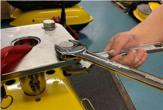
*Figure 4-53: 3400 Light and Ultra-Light Adaptor Flange Plate Bolt Assembly - Bolt Tightening*
