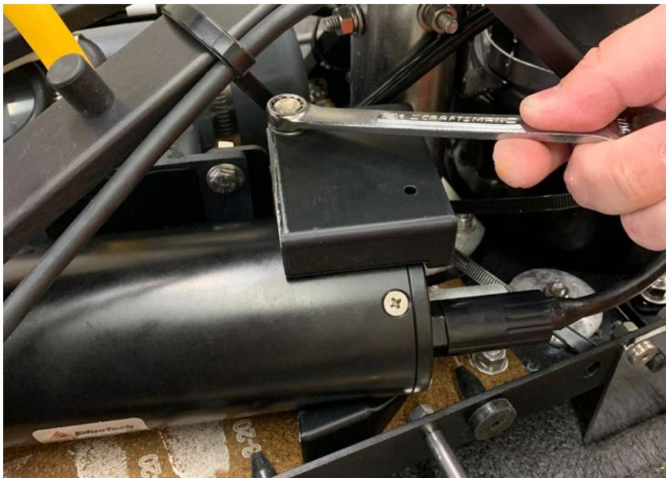
*Figure 5-16: 3400 OTS Light and Ultra-Light Mounting Block Bolts*
