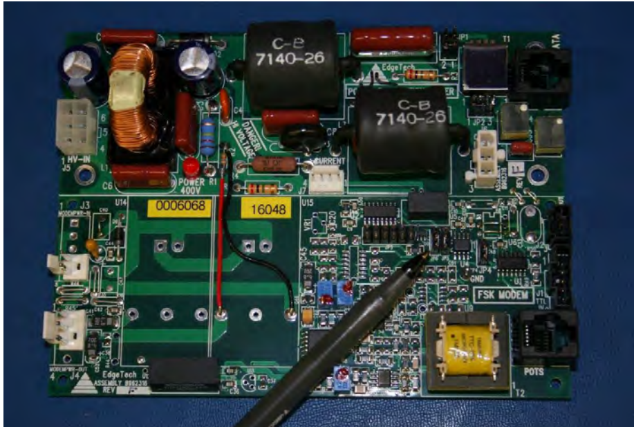
Figure 4-1: Location of Jumper JP6 on the Power Board of the FSIU
