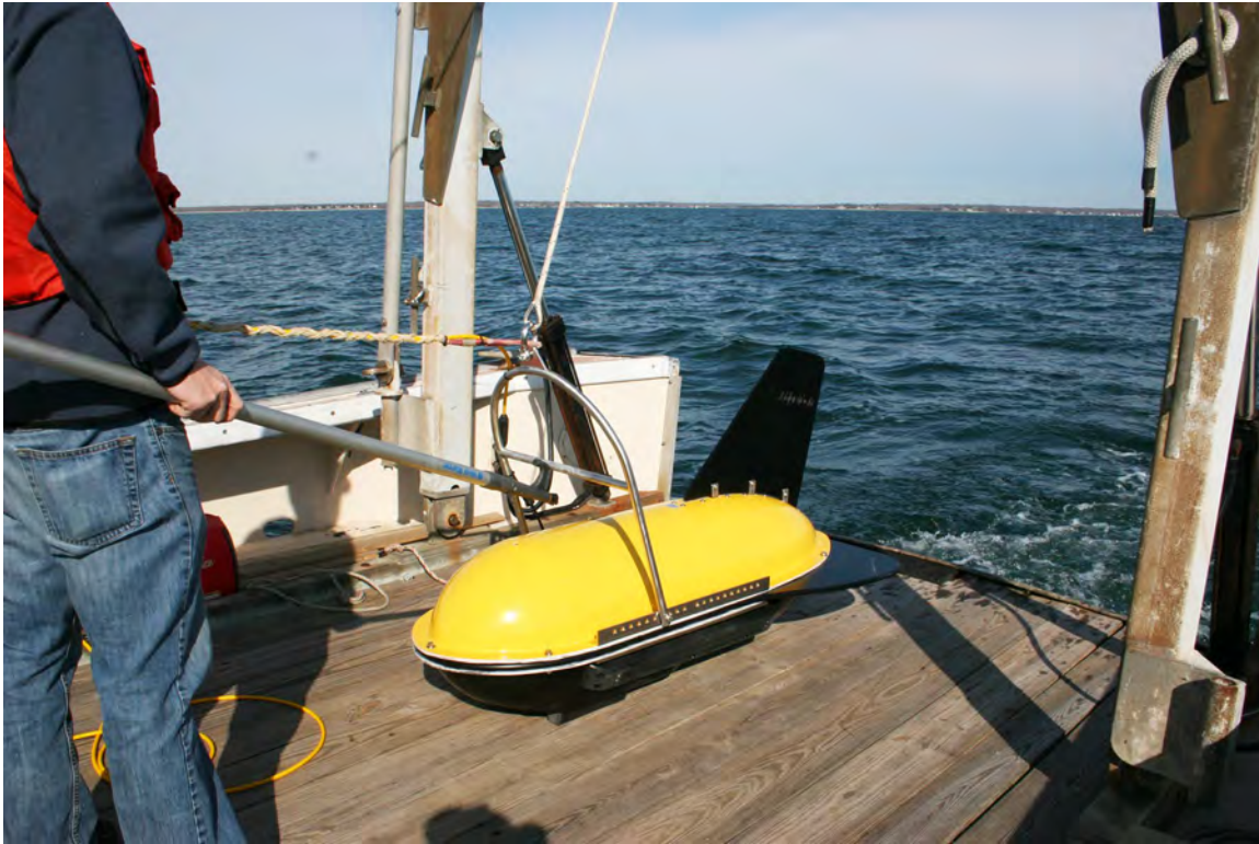
Figure 1-1: 2000-DSS Tow Vehicle being Prepared for Deployment
