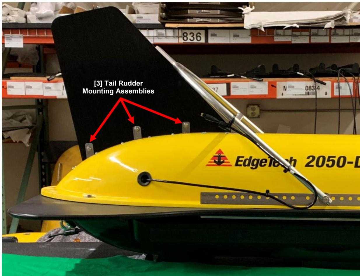
Figure 5-1: 2050-DSS Tail Rudder [3] Bolt Hardware Assembly Locations
