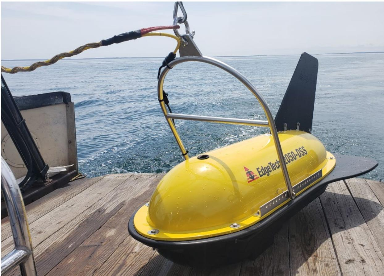
*Figure 4-18: 2050-DSS Tow Cable and Grip Bridle Attachment*
