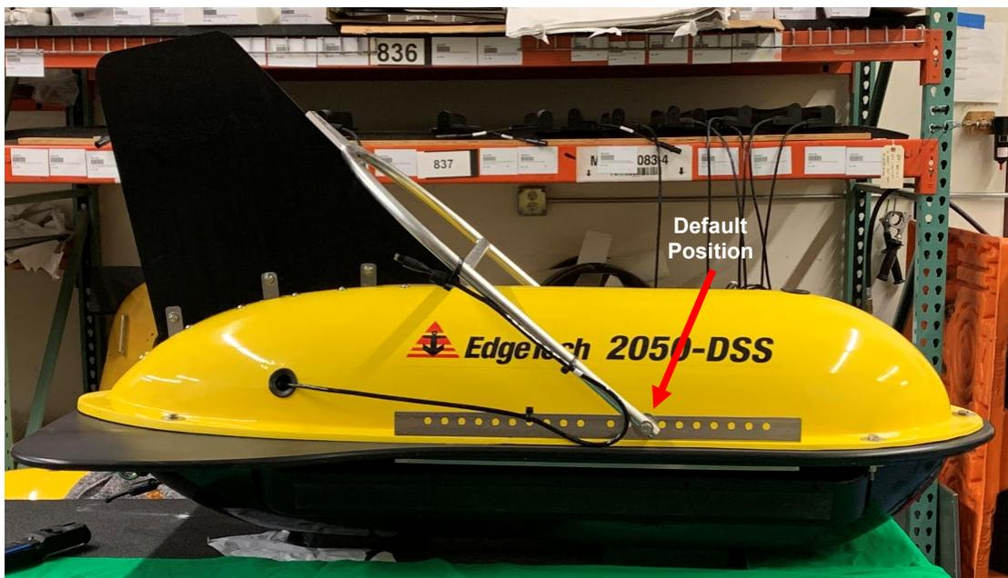
*Figure 4-15: Tow Fish Bridle Mounting Bracket Positioning*
