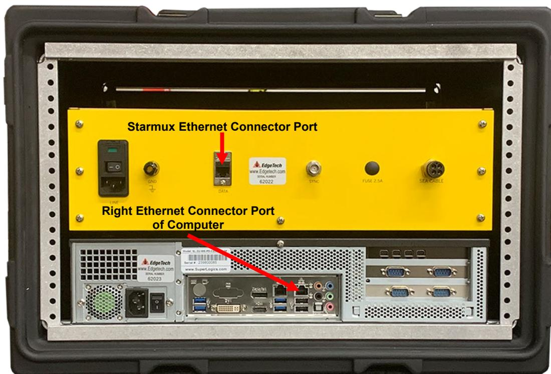
Figure 4-1: Starmux IV and Computer Connected By Ethernet Cable
