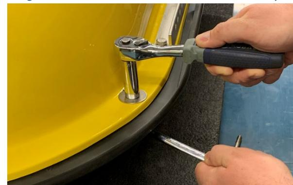
*Figure 5-5: 2050-DSS Bolt Hardware Disassembly*
