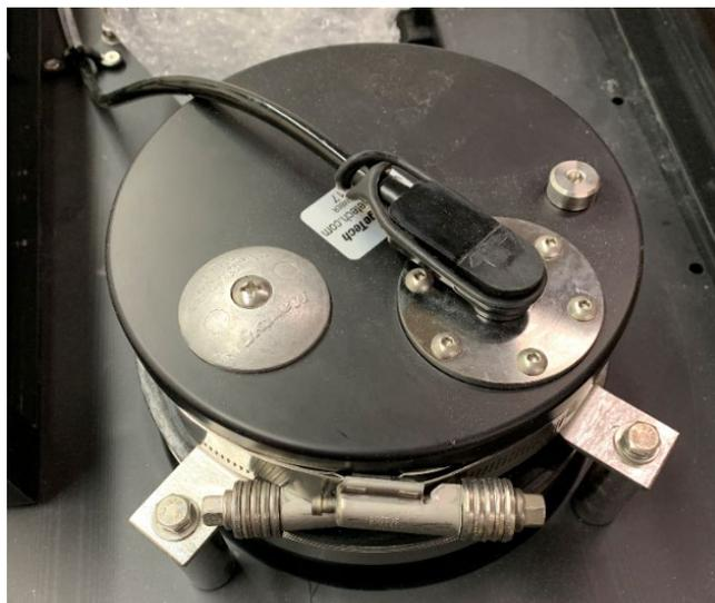
*Figure 5-9: 2050-DSS Sub Bottom Transducer Clamp and Mount Orientations*
