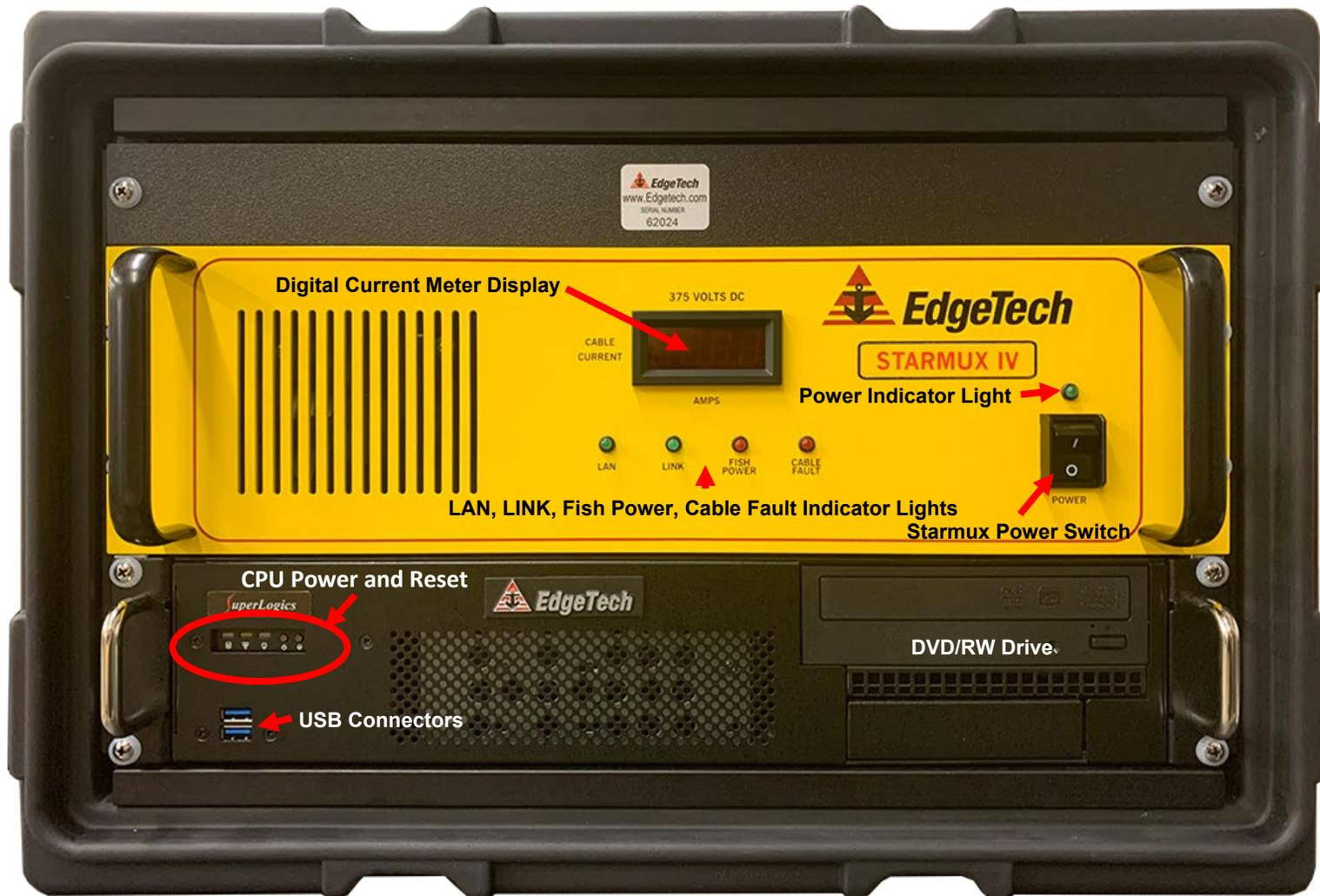
Figure 3-8: Labeled Front Panels of Starmux IV Rackmount
