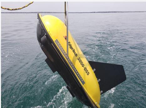
The EdgeTech 2050-DSS is the latest product to combine EdgeTech's highly successful line of side scan sonars and sub-bottom profilers into one fully integrated system. This is especially useful where high resolution sub-bottom profiler data, that requires the system to be towed near the seabed, is required.
