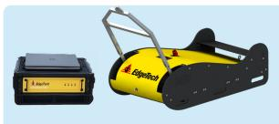
The system generates high resolution images of the sub-bottom stratigraphy in oceans, lakes, and rivers and provides excellent penetration in various bottom types. The EdgeTech 3400 comes in a dual 2-16 kHz transducer configuration. The towfish is configured with new PVDF receiver arrays segmented for standard sub-bottom profiling operations or a unique "pipeliner" mode for optimal location and imaging of buried pipelines.
