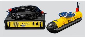
This unique Hybrid approach utilizes multiple receive arrays and combines both Beamforming and Phase Differencing techniques to determine each sounding along the seafloor. With the integration of EdgeTech's Full Spectrum  $^{\circledR}$  CHIRP technology, the 6205  $^{\char{red}{S2}}$  exceeds IHO SP-44, NOAA, and USACE specifications for Feature Detection and Bathymetric Point Data Uncertainty.
